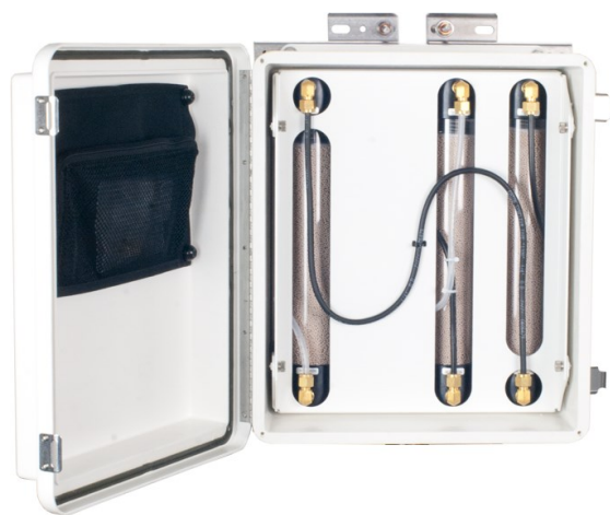
Figure 4-14. Interior of CPEC310 scrub module
