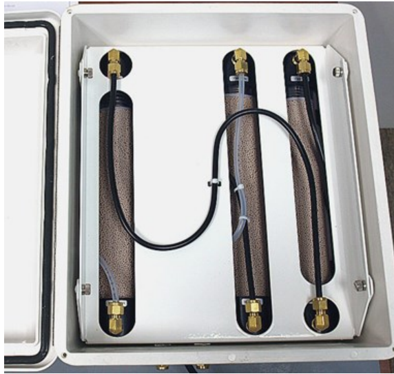
Figure G-2. CPEC310 scrub module interior
